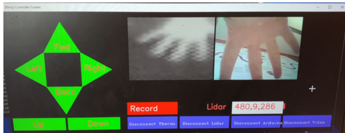
Figure 3: User interface: Green buttons control the blimp's movements, blue buttons start threads to read sensors, and the red button enables recording. The text field shows LiDAR distances, and the videos show thermal (left) and RGB data (right).
